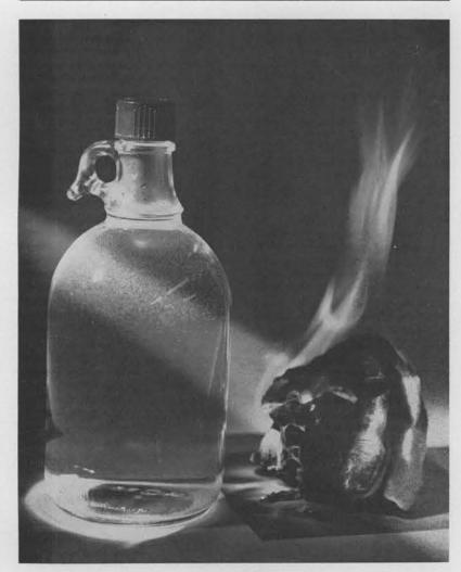
FIRE HAZARD—This innocent looking bottle of clear liquid becomes a fire hazard when rays of the sun passing through it are refracted as in a magnifying glass. Resulting heat can cause flames.
